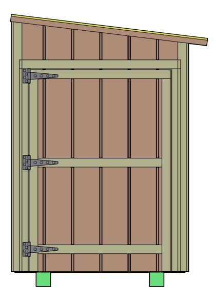
This is an end view of the 6ft low profile bike shed. It's designed to sit flush right up to a wall. Or you can put overhang on both sides for a free standing shed.
