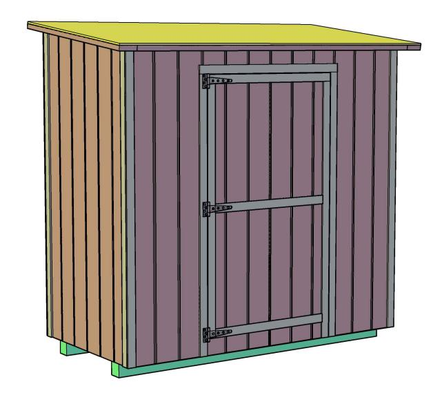
Same 4x8x8 tall shed with the door on the low side and no overhang on back so you can sit it flush against a wall.
