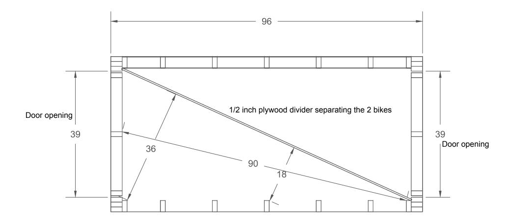
This shed has a door on either end. Back your bike in and the plywood divider guides it in at an angle to keep it separate from the bike on the other side.
